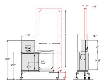
Representational Drawing. Request drawing specific to your application. The ROMS-4/TRS-4 strapping machines are built-to-order machines and can be configured in a number of track sizes. See chart for available combinations.
